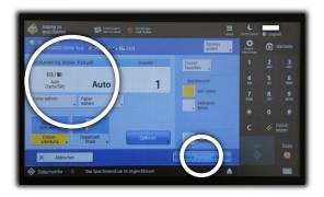
Set the desired **options\*)** and confirm with "**Druckstart"** (Start printing).
